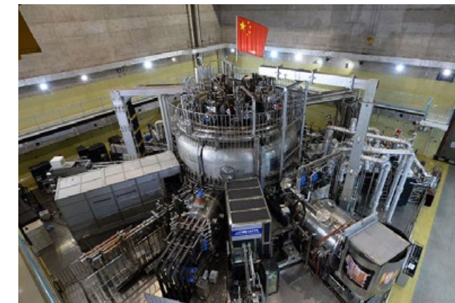
■ Tokamak HL-2M du Southwestern Institute of Physics - Source : Yicai Global
